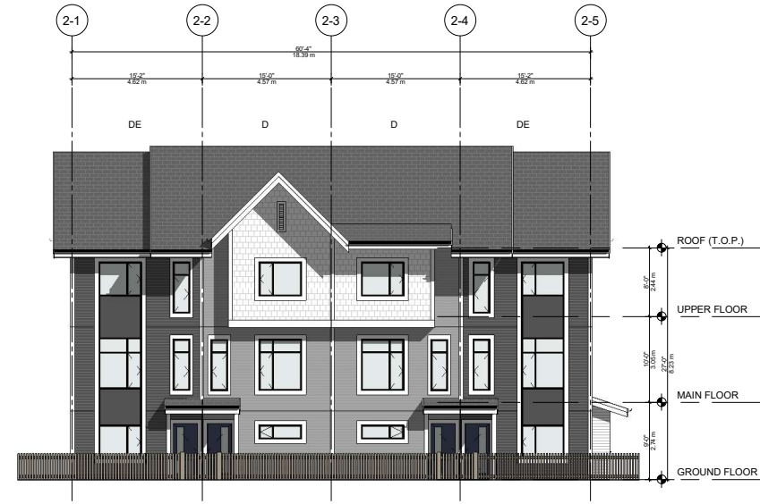
1 SOUTH ELEVATION - BUILDING 2 & 17 1:100
